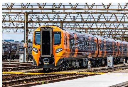
**Our new Class 196 fleet of diesel trains are nearing entry into service on the Shrewsbury Line.**
